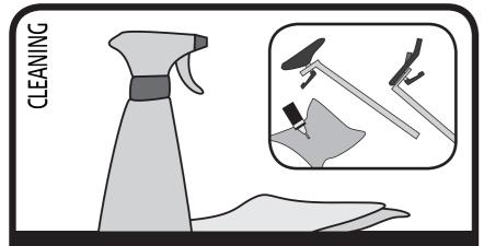
After each workout, wipe the cycle down with tissue paper. Every other week the posts need cleaning to protect them from sweat etc. Pull out the seat post and the front post and wipe them clean with an oily cloth.
